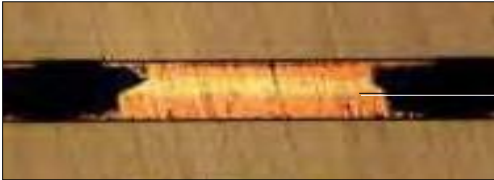
Image of the bond between wafer pairs
